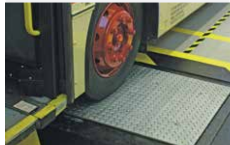
VLTPWD9143 wheel play detector (74) max axle weight 20000 kg stroke 100 mm remote control with lamp
