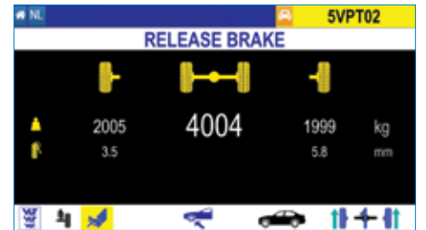
starting measurement prior to brake test
