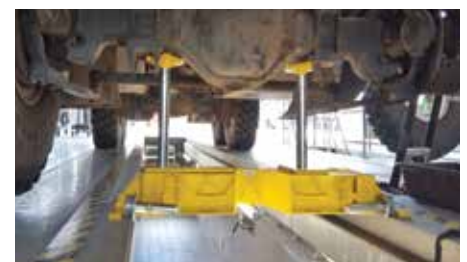
BPJA-AFZB15 Supporting bridge
